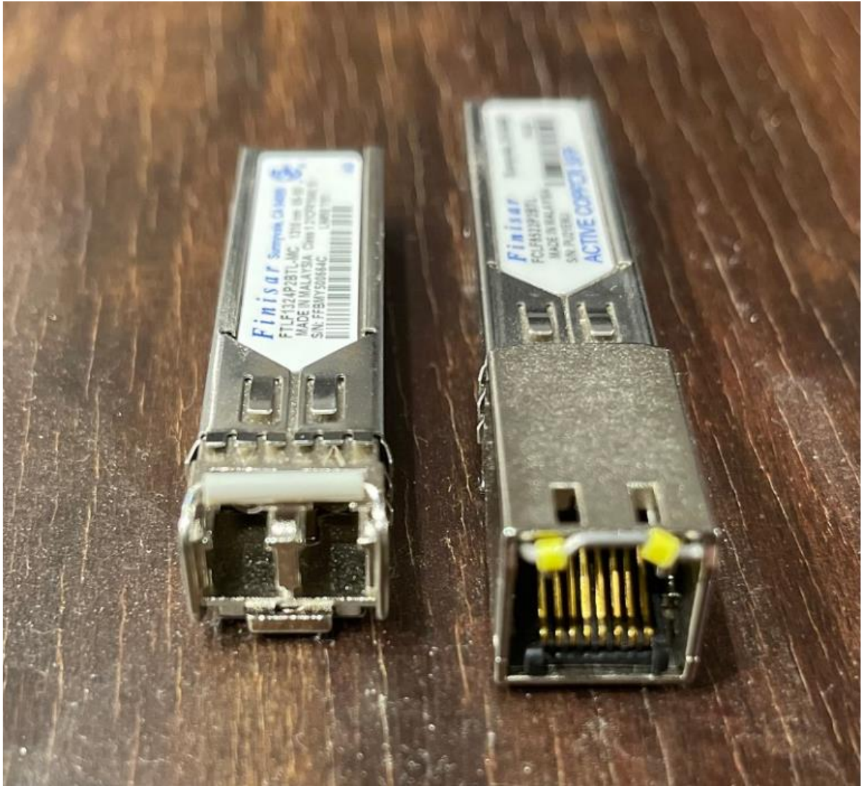
Above is a photo of a fiber and a copper SFP RJ45 module
